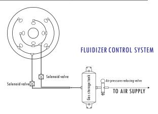
Effective placement of aerators depends on material type and volume requirements.
